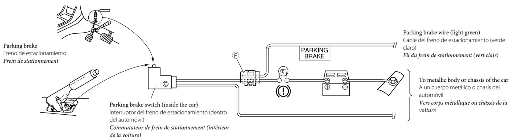
**When installing the monitor in a location where it cannot be seen by the driver**
