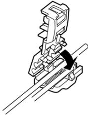
Contact the metallic part of the crimp to the wires inside.
